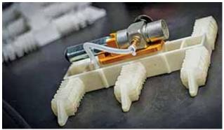
This robot can walk, without electronics, and only with the addition of a cartridge of compressed gas, right off the 3D-printer (Credit: David Baillot/ University of California San Diego)
